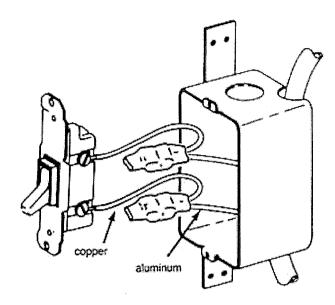
Reconnection for typical feed-through circuit with AMP COPALUM Connectors.
